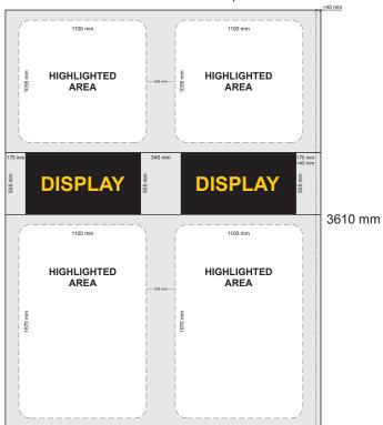
Please note: the white broken line indicates where the artwork will be cut and attached to the perspex on the column. This area is referred to as the safe copy area and placing small copy over this line should be avoided as there is a 10mm lip.
